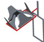
Grab/pull device used to secure material
